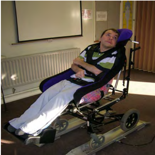
Figure 3. Client being weighed using wheelchair beam scales
